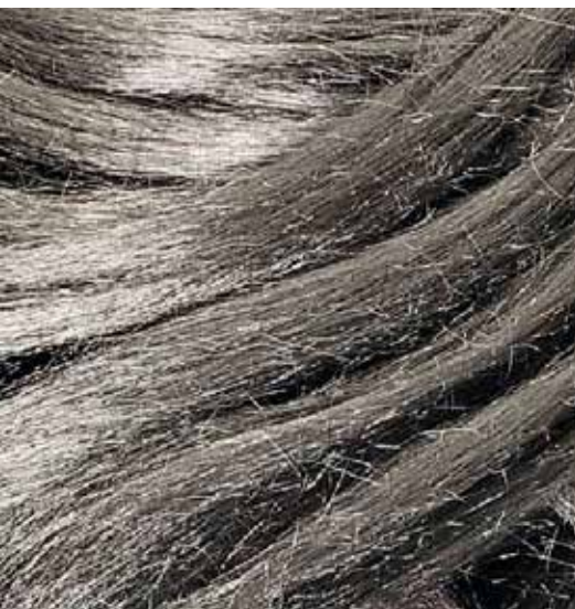
Bekaert Bekinox® VS stainless steel fibers for the textile industry
